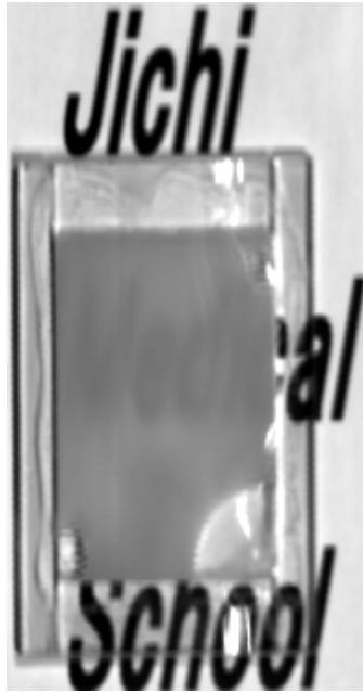
Fig. 2. Visualization image of wavelength 1100nm, printed-paper and blood layer with 3mm
