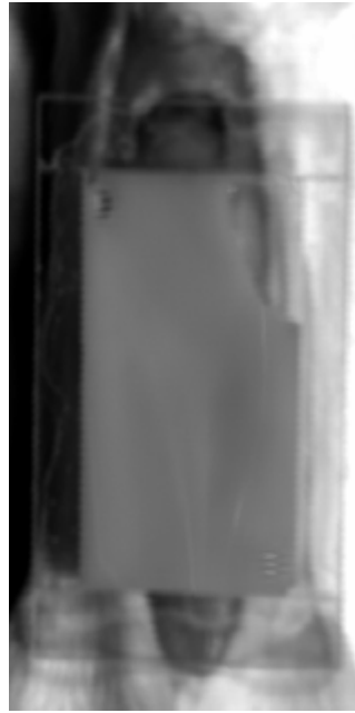
Fig. 4. Visualization image of wavelength 1100nm, guinea pig opened abdomen with viscera shown, covered with a blood layer of 3mm thickness
