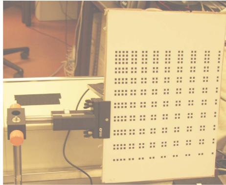
**Figure 3.** The calibration grid mounted on the optical table
