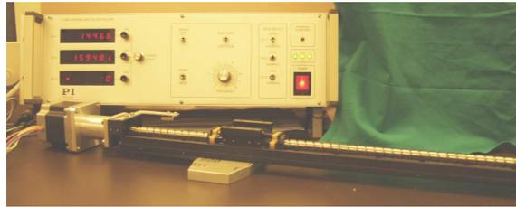
**Figure 5.** Stepping motor controller from PI and linear positioner.
