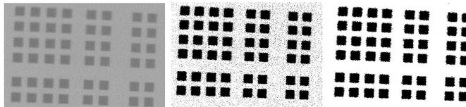
**Figure 4.** The first figure shows the image provided by the CCD camera, in the second figure the image is thresholded, the third figure is made after removing the smaller objects caused by the image noise. The next steps are calculating the centers of gravity, detecting the *x* and *y* axes and at last the points can be associated to their coordinates using the cross value.
