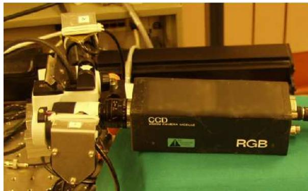
**Figure 1.** A photograph of a prototype of the Varioscope AR. At the ocular of the base instrument a CCD camera was placed.
