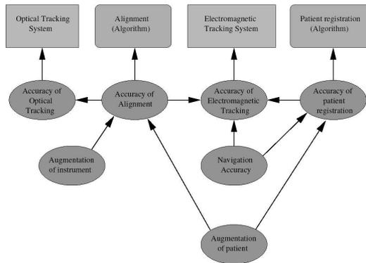
**Fig. 5.** Errors, induced by the different tracking systems and registration procedures. Arrow direction means 'depends on'.
